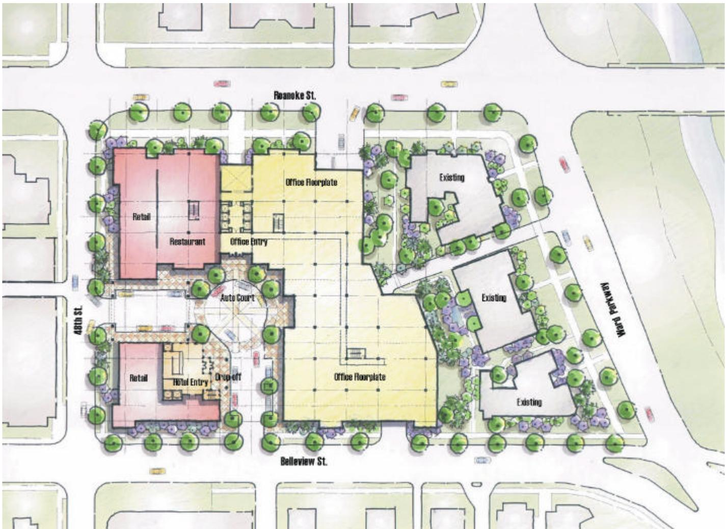
Above is an architect's drawing of the latest version of Ray Braswell's proposal. North is to the left. The drawing is of the ground level for the block. The proposed hotel would be above the retail space, facing 48<sup>th</sup> Street. The main entrance to the parking is from Roanoke. The three existing buildings would have access to the parking via the drive from Ward Parkway.
